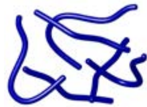
Polymer Damaged By Excessive Mixing
